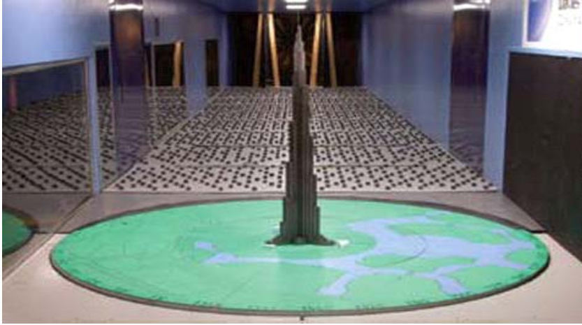
Fig. 4 Wind tunnel model at the Boundary layer wind tunnels at Guelph, Ontario, Canada (Source: Ref. 5)
