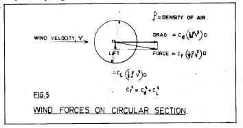
For circular and rounded sections, force coefficient  $C_f$  vary with Reynolds number since the point at which the flow becomes turbulent is controlled in part by the velocity, whereas for angular sections such as squares and triangles, force coefficients are independent of the Reynolds number, and are wholly determined by the angularity of the shape.
