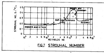
have been made for values of R more than  $10^7$  in view of the difficulty in relating model test results to full scale structures. The draft revision to IS: 875-1964 suggests a Strouhal number of 0.25 which if finally adopted will have a significant effect in the dynamic analysis in that resonant moments will be reduced by 36 per cent from those corresponding moments calculated S=0.2.
