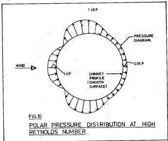
Reynolds number. The Indian Code IS: 4998 gives an emperical formula for the calculation of bending moments in the horizontal plane for a circular shaft considering these pressure variations, and the Code also recommends minimum shell thickness in relation to the chimney diameter to avoid ovalling effect.
