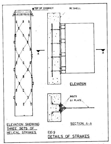
Many chimneys, both single flue chimneys and the multi-flue type, in the country have been provided with such strakes at the advice of the Indian Institute of Science, Bangalore, following their model testing in wind tunnel.
