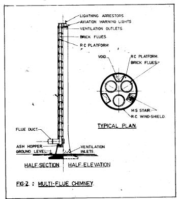
multi-flue chimney generally serves only one boiler, and thus they are not affected by high ratios of maximum to minimum loading fluctuations. Although the cost of multi-flue chimney is usually more than that of the single flue type of a similar flue area, but it has its own advantage in operation and maintenance. Many multi-flue chimneys, height ranging from 160 m to 225 m height, have been built in the country in recent years for super thermal power stations.
