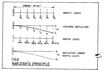
the assumed deflection should be close to that of the calculated deflection shape. For higher mode frequencies, a stiffness matrix method using computers can be used with great speed and accuracy.
